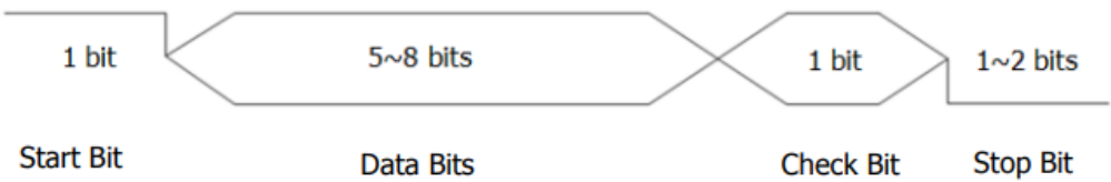
Figure 8.13 Schematic Diagram of UART Protocol
