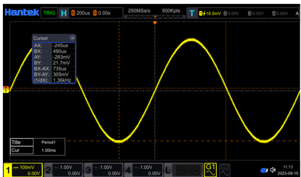
Figure 10.4 Track Measurement (after Horizontal Expansion)
